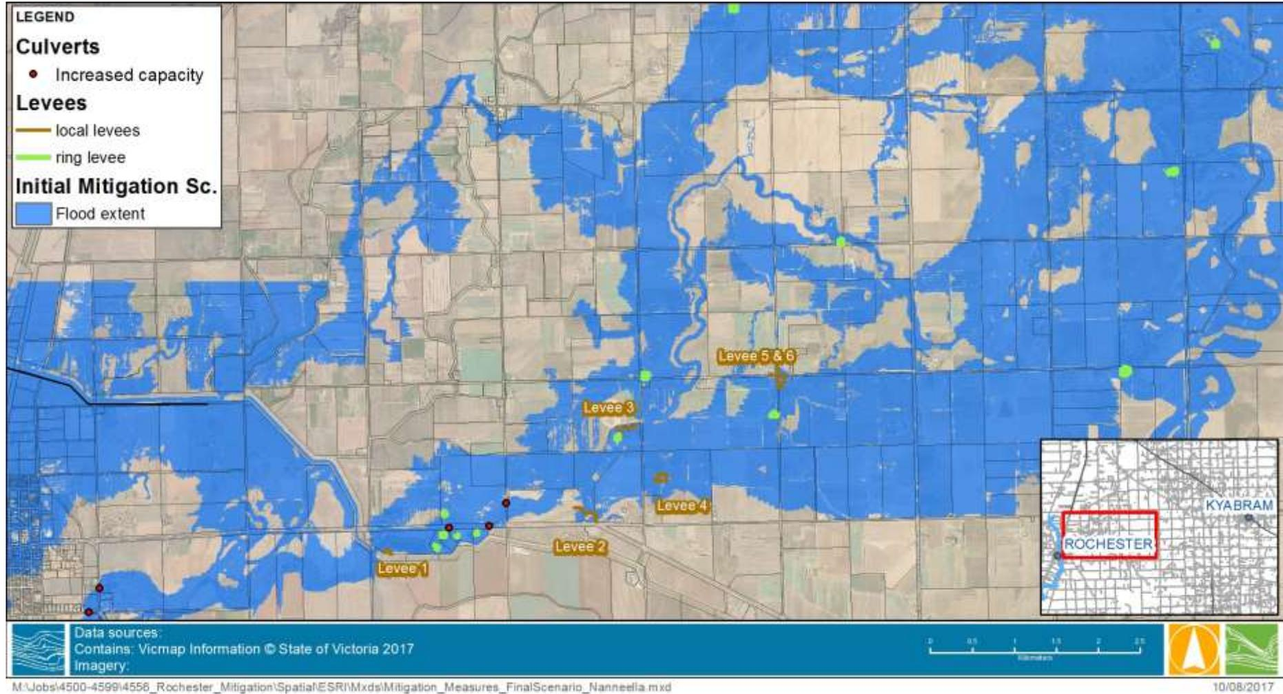
FIGURE 8-2 FINAL MITIGATION SCHEME KEY FEATURES – NANNEELLA DEPRESSION
